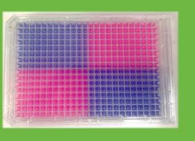
HTS requires robust assays that repeat 1000's of times. The Z' assay tests this repeatability by using 3 full plates ½ positive control and ½ negative controls in a quadrant pattern. The signal window and variability measure calculated must be >0.5 and <1. our PD-1 assay produced Z' = 0.78.
