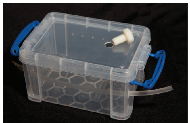
Figure 1. Modified Really Useful box for housing spiders of medical importance, showing feeding aperture in the lid (with closure bolt) and CO 2 line for anaesthesia.
